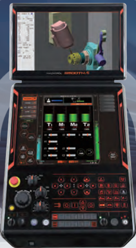
Shown with optional MAZATROL SmoothAi dual monitor
