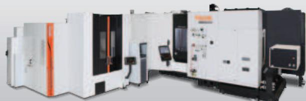
PALLETECH with Horizontal Machining Center
