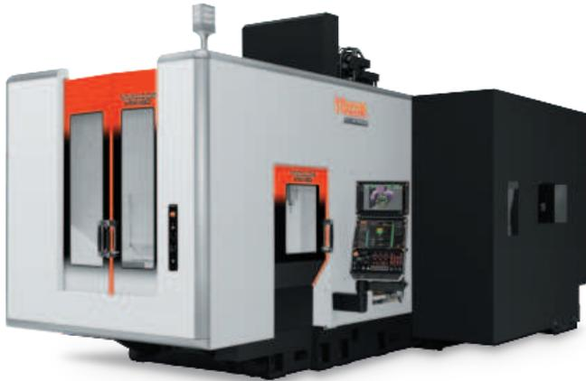
For higher productivity, set up the next workpiece during machining of the current workpiece. The 2-pallet changer offers a compact design and is suitable for mass production. Reduced length to pull out the rear conveyor saves space in the maintenance area.
