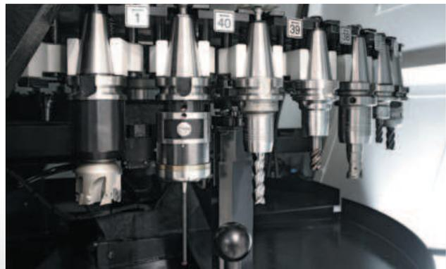
The standard tool magazine accommodates 30 tools, with 40, 80 and 120-tool options available. This generous capacity provides ample storage for complex workpieces and high-mix production, as well as spare tools for prolonged continuous operations.
