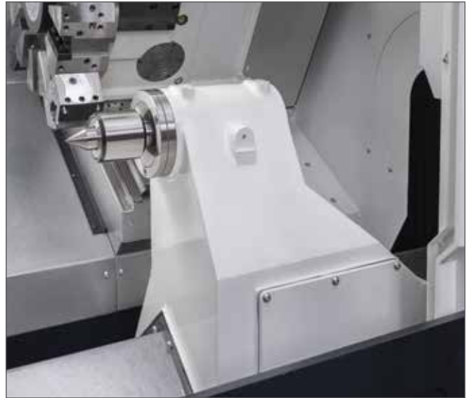
NC SERVO-DRIVEN TAILSTOCK
