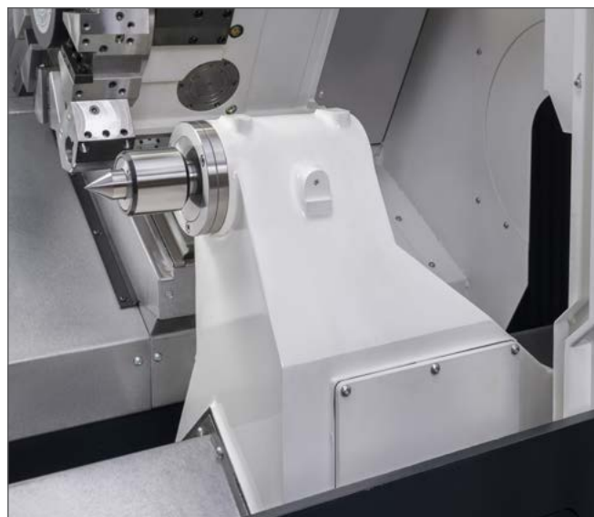
NC SERVO-DRIVEN TAILSTOCK
