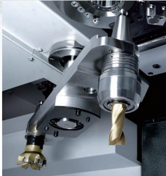
Our high-speed ATC system employs a simple and reliable servo driven cam actuation system that aids in rapid tool change to reduce non-cut time. Spindle utilization is also increased through bi-directional rotation of the magazine to the next required tool position, bringing more productivity to your facility.
