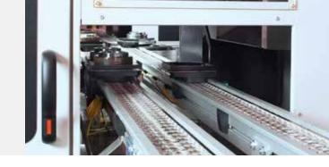
Made for increasing productivity, throughput and quality when turning shaft-type parts, a bar feeder is one of the simplest, most cost-effective forms of automation available. It allows you to automate the loading and feeding of bar material into your CNC lathe with minimum built-up area required. Standard bar feeders typically feed bar material up to four inches in diameter, but if you need a larger size, we can help with a custom solution.
